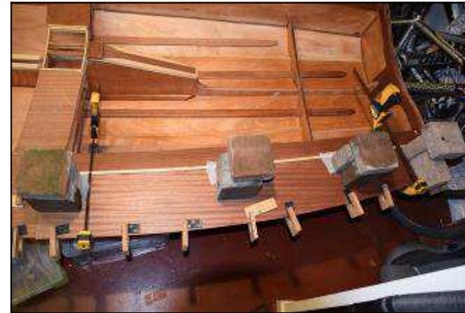
The rear decks are clamped and weighted with bricks while the epoxy sets
