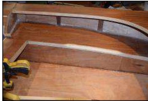
The whitewood strip is glued in place and the crew seats have been faired off with an angled cut out to mount the jib cleat tracks on
