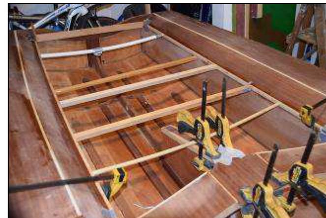
The rear decks have been faired off and grab rails are glued into place neatly hiding the join between deck and side tanks. To avoid screwing or pinning them they are wedged with lengths of scrap wood.
